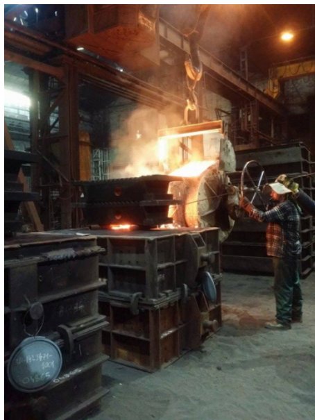
Figure 2. Casting into casting boxes. Due to oxidation and evaporation under atmospheric conditions, the effects of the preconditioning agent slowly disappear.
