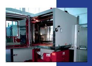
O cooling-heating speed 15 degrees/min.
